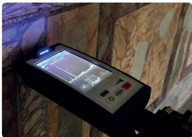
BRAVO™ Raman analyzer investigating a fresco
