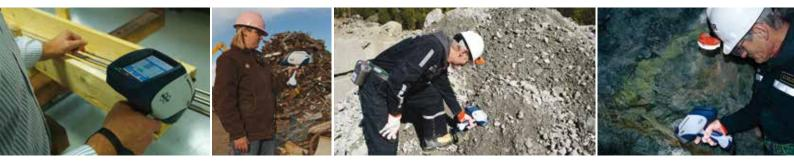
**Detector Technology:** The S1 TITAN can be configured with either the performance-based Silicon Drift Detector (**SDD**) or the economical Silicon PIN Diode (**SiPIN**) detector.
